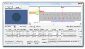
script, see an exposure in relation to other exposures, and a crude preview of what it will look like. The graph at the upper right plots exposures over time, with vertical axis height plotting each exposures' "Q", or absolute exposure setting (factoring in shutter speed, aperture, and ISO). Black boxes show when the shutter is actually open, with red tails representing the 'Recycle Time', which is how long before the camera is ready to take another exposure.
