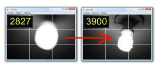
fantastic tool to achieve pinpoint focus on Eclipse day. Select 'Window | Live View' from the main menu bar, then pick your camera from the 'Camera' menu in the Live View window. You can optionally turn on the Sharpness metric and grid lines. The higher the number, the sharper the image. For best accuracy, we recommend selecting 'Settings | Zoom In'
