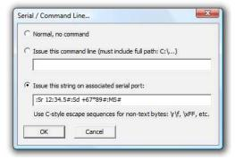
command a Meade LX200-compatible telescope to slew to a right ascension of 12h 34.5m and a declination of +67°89'.
